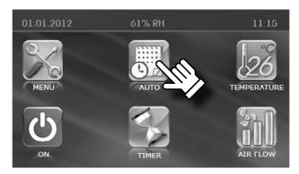
• The **AUTO** mode enables scheduled operation of the ventilation unit. The unit runs at the preset speed and temperature during the specified time periods.
