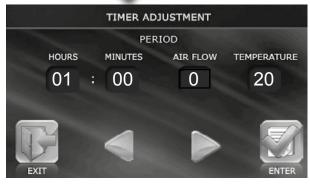
• To activate the timer, press **TIMER** in the control panel Main menu.
