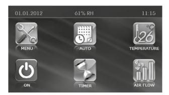
The Main menu contains the date, current humidity, time, temperature and set air flow. This menu also works as a hub for accessing the main control panel functions and menus.
