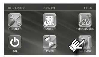
• Press the AIR FLOW button to select the desired fan speed.
