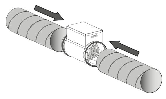
The heater is designed for internal installation into air ducts in the horizontal or vertical position. In a horizontal position the connection box must face upwards. Permitted deviation up to 90 °C. The heater must not be mounted with the connection box suspended downwards (risk of condensate leaking and short circuit of power grid).
