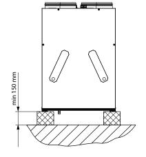
Note: mounting is shown by the example of the KOMFORT EC S(B)200(-E) unit.
