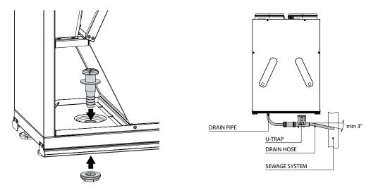
Note: installation of the drain pipe is shown on the example of the KOMFORT EC S(B)200 unit.
