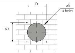
3. Insert the supplied expansion anchors 6x40 into the holes. Remove the outer ventilation hood to enable access to the fastening holes. Pull the front part below toward you.
