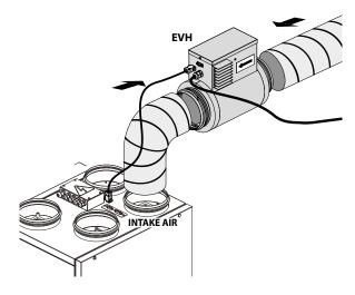
Heater position In case of horizontal mounting position the control box cover must be directed upwards only. The maximum deviation angle is 90°. The control box cover may not be positioned downwards!
