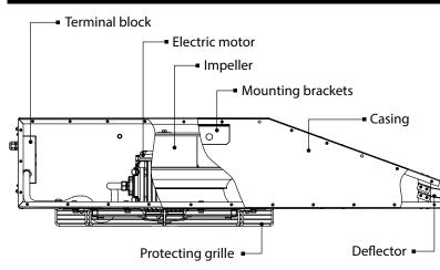
The fan casing is made of polymer coated steel. The protection grille on the air inlet side prevents ingress of foreign objects. The deflecting plates on the pressure side ensure equal air distribution and boost air draft.
