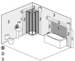
CAUTION! The unit must be installed at a distance of at least 2.3 m from the floor.
