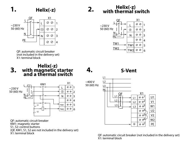
Wiring example for the **Helix(-z)** fan with external leads of the motor overheating protection and a magnetic starter is shown in Fig. 3. The terminals **TW1**, **TW2** are the leads of the normally closed contact of the motor overheating protection.
