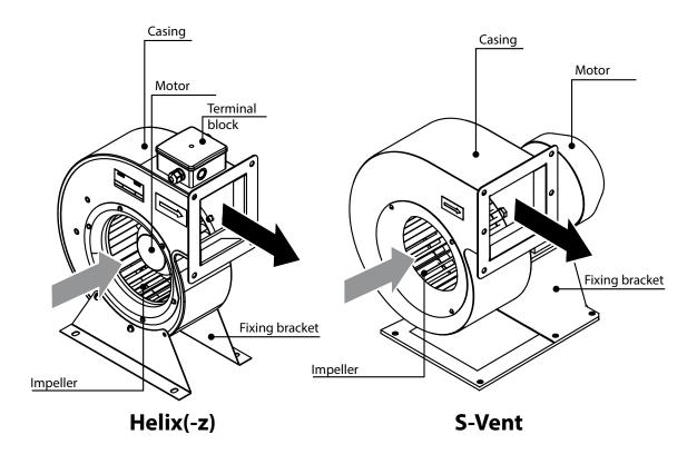
The **S-Vent** fan is enclosed in a metal casing. The electric motor and the air intake ring are fixed to the casing through the flange. The impeller is fastened to the drive shaft.
