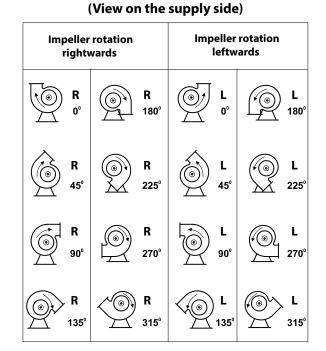
**POSSIBLE VARIANTS OF THE S-Vent FAN CASING POSITIONS**
