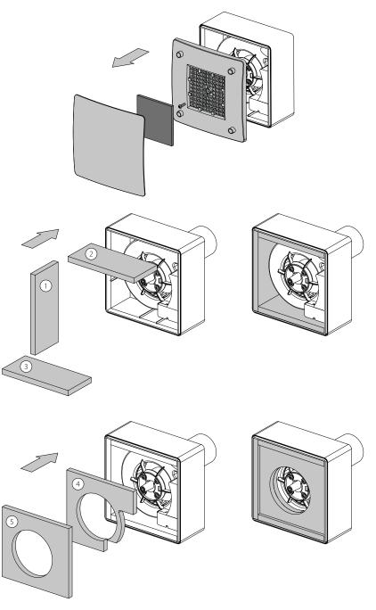
2. Install the parts of the sound insulation kit one after another as shown in the figure.
