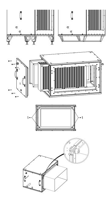
If the cooler is to be mounted on the floor, the feet must be screwed on.
