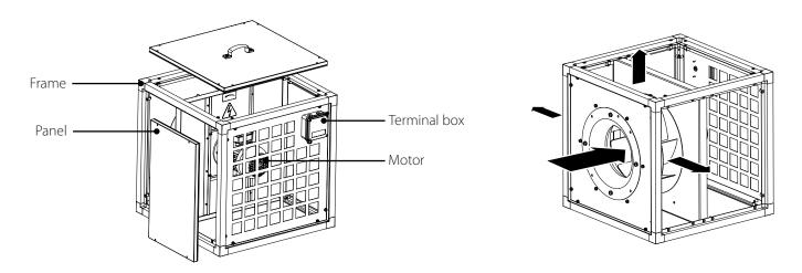
When connecting the fan to the air duct system, it is recommended to use the accessories specified in the User's manual. Connecting spigots can be of round cross-section.
