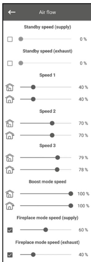
This menu section enables setting the air flow values for the **Standby** mode, speed 1,2,3 pre-sets as well as the **Boost** and **Fireplace** modes.
