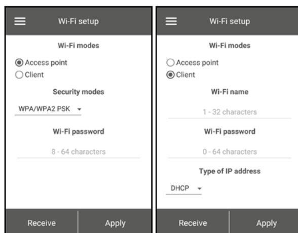
**Access point:** access point mode without a home router. Up to 8 devices can be connected to the unit in this mode.
