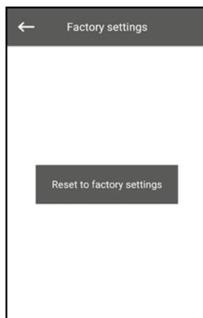
Use this menu to revert all the settings to their factory values. The reset may cause a temporary loss of connection to the device as it affects the Wi-Fi, RS-485 and Ethernet settings. If necessary, enter the new settings for your Wi-Fi, RS-485, and Ethernet connections.
