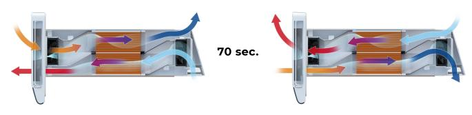
The regenerator is divided into two parts, which are isolated from one another, thus eliminating the transfer of heat and moisture between them. One of the fans operates in the supply mode: fresh cold intake air from outside flows through the first regenerator, and absorbs the accumulated heat and humidity.
