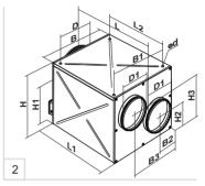
Overall and connecting dimensions of Iso-ZS fan with two intake spigots and one exhaust spigot
