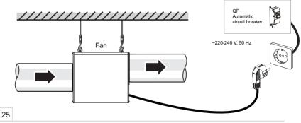
Wiring diagram for connection of Iso-ZS fan to AC power mains via a power cable and a plug
