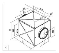
Overall and connecting dimensions of Iso-ZS fan with one intake and one exhaust spigot
