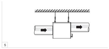
Iso-ZS fan mounting and operation example
