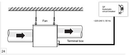
Wiring diagram for connection of Iso-ZS fan to AC power mains via a terminal box
