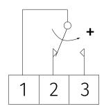
Humidification Dehumidification Closing contact between terminals 1 and 2 Closing contact between terminals 1 and 3
