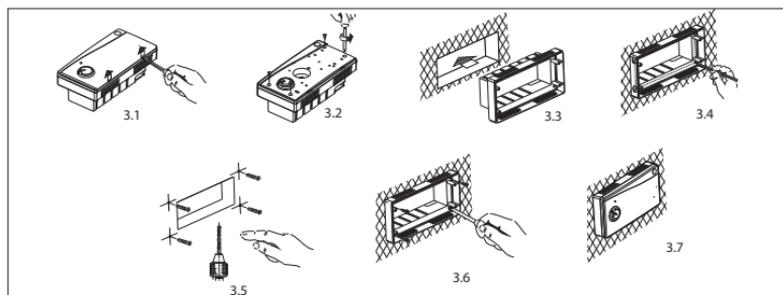
Fig. 3. TI/HSI/LSI/IRSI mounting
