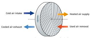
Rotary heat exchanger operating logic
