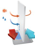
The **KOMFORT Ultra L250-E S12 (white)** unit is equipped with a plate enthalpy cross-flow heat exchanger made of polymerized cellulose that recovers heat and humidity. Due to humidity recovery the enthalpy heat exchanger produces no condensate.
